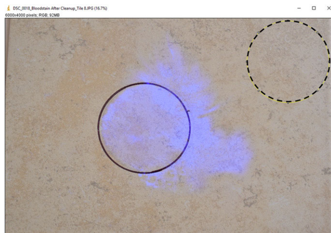
FIG. 1—Selection of ROI in ImageJ, represented by the dotted line; three such ROIs were measured for each tile; the solid line represents the original location of the blood droplet.
